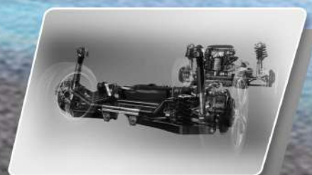
FRONT MCPHERSON & REAR MULTI-LINK INDEPENDENT SUSPENSION
